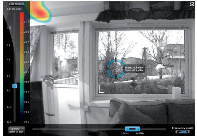
Having determined that the intake valve was the main noise contributor, this spot was covered up with a pillow to remove it from the overall noise field, and try to locate secondary sources. By filtering on a relatively high frequency band around 3 - 4 kHz, it was possible to filter out only the noise being emitted by small gaps and cracks. This produced two new possible weaknesses, one on the porch door, and another on the air valve above the window as seen in the image below.
