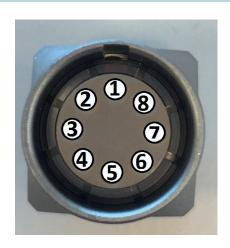
Figure 5: Weather station connection. Terminal block (left), and Lemo connector (option 1 - right)
